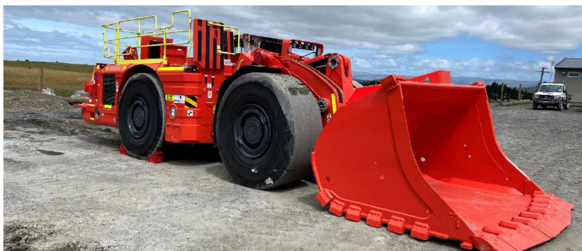
New Underground Loader, a Sandvik LH517i, at the Macraes Operation in New Zealand. This machine has a low emission engine and onboard intelligent control system.
